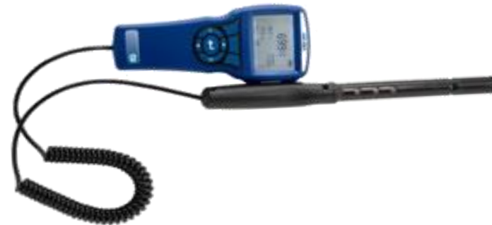
CO 2 , temperature and relative humidity monitor (IAQ-CALC monitor model 7545, TSI Inc., MN, USA)
